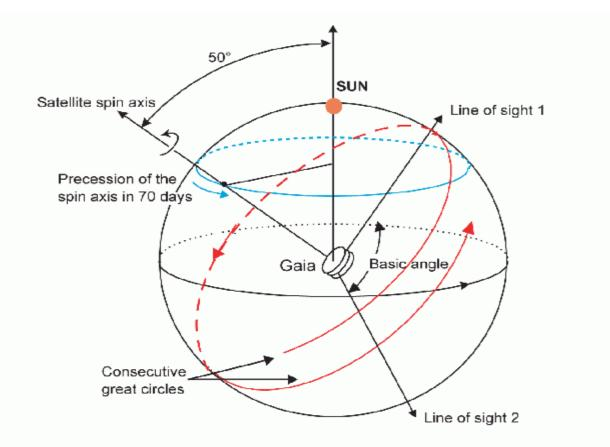
Gaia's two astrometric fields of view scan the sky according to a carefully prescribed 'revolving scanning law'. The constant spin rate of 60 arcsec/s corresponds to 6-hour great-circle scans. The angle between the slowly precessing spin axis and the Sun is maintained at  $50^{\circ}$ . The basic angle is  $99.4^{\circ}$ .
