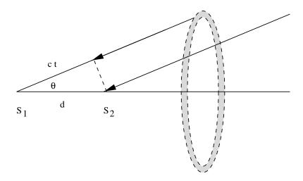
The time difference t between arrivals of the burst at spacecraft  $S_1$  and  $S_2$  gives the angle  $\theta$ , from  $d\cos\theta = ct$ .
