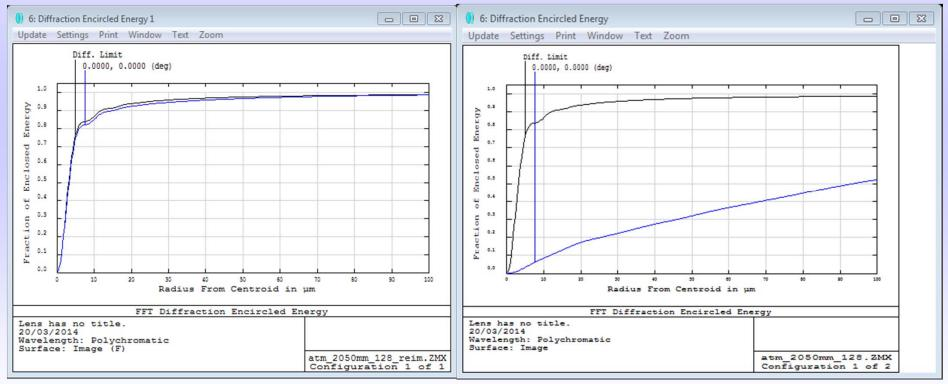
In this simulation the correction of the two layers is limited by the correction out of the pupil plane, phase is so large that rays are out of the field
