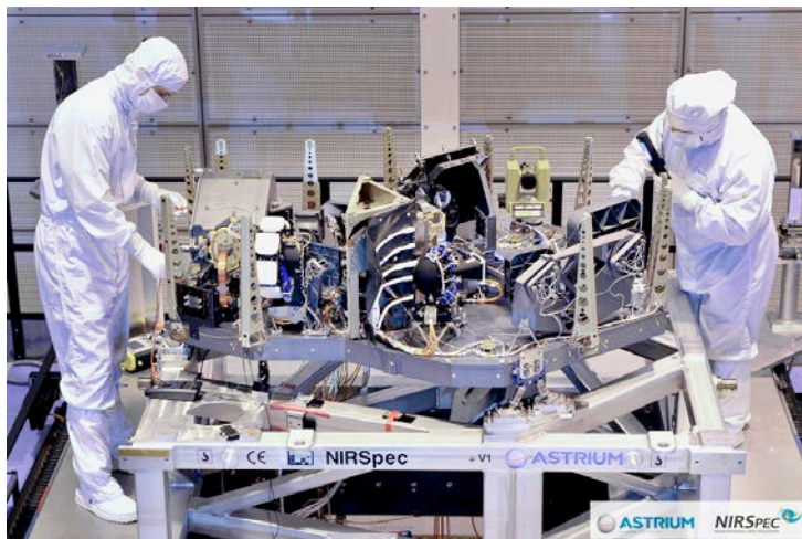
JWST/NIRSpec - FM2 cryogenic test campaign 01/2013
