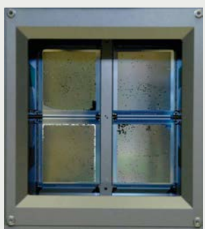
MEMS device – 105x204 micron shutters
