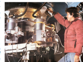
Figure 1. — A youthful Tetsuomi tops up the liquid nitrogen A UKT6 at the Cassegrain focus of UKIRT (c. 1982). UKT6 can be seen to its left. (Image courtesy Royal Observatory Edinburgh.)
