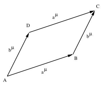
Figure 7: Consider parallel transport of a vector around the anticlockwise loop ABCD. It suffices to consider a parallelogram, as any general loop can be made up from a collection of such elements. The overall change in the vector is the change over the path ABC minus the change over the path ADC.
