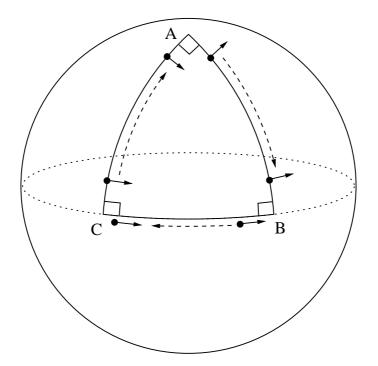
Figure 6: This figure illustrates the parallel transport of a vector around a closed loop on the surface of a sphere. For the case of the spherical triangle with all angles equal to  $90^{\circ}$ , the vector rotates by  $90^{\circ}$  in one loop. This failure of vectors to realign under parallel transport is the fundamental signature of spatial curvature, and is used to define the affine connection and the covariant derivative
