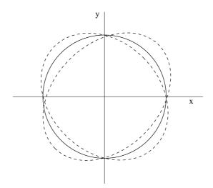
Figure 9: Effect of gravitational wave with  $\times$  polarisation.
