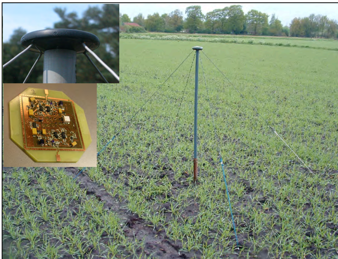
Low band antenna: 30 – 80 MHz 48/96 antennas per station
