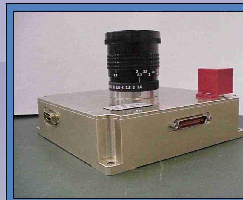
4a. Interior view of the NPAL navigation camera showing the image processing chip (red box). 4b. Exterior view of NPAL navigation camera.
