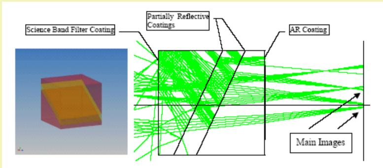
Figure 7.1: HOCS Optical Element and Ray Trace
