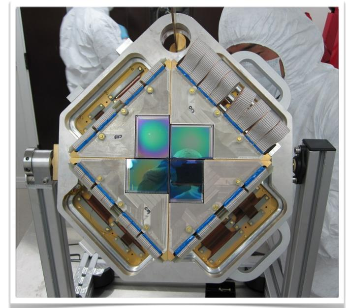
450  $\mu$ m focal plane unit prior to installation
