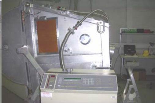
Photo 12: 4K assembly leak check.
