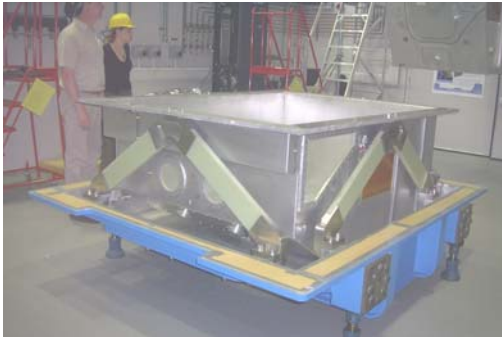
Photo 11: 60K to VVFS via large truss assembly.
