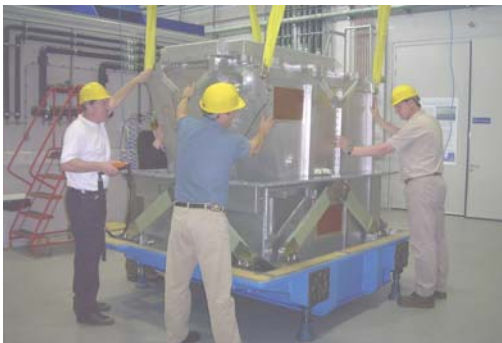
Photo 13: Trial integration of 4K stage via small truss assy.
