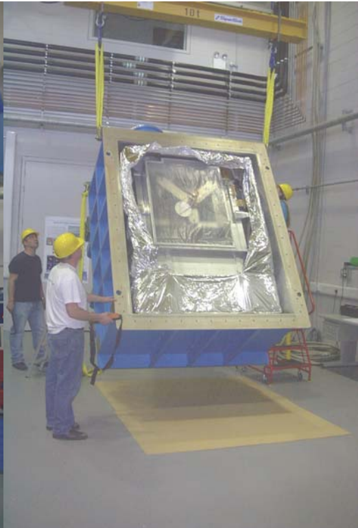
Photo 16: VVMS integration complete (note cold shutter).
