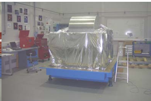
Photo 16: Real integration complete with MLI blanket.
