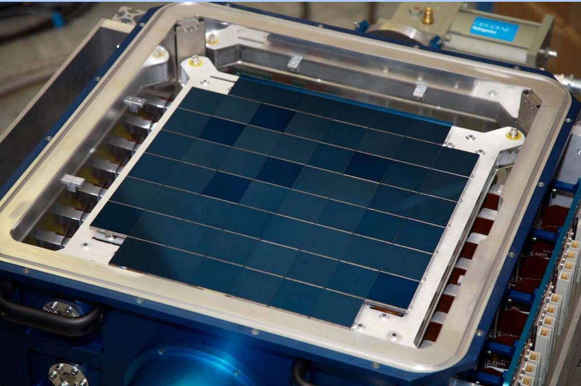
One of four 1.4 GigaPixel camera for the Pan-Starrs project using a new CCD design.
