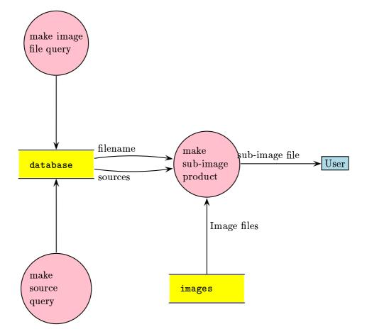
Figure 8: Image extraction data flow
