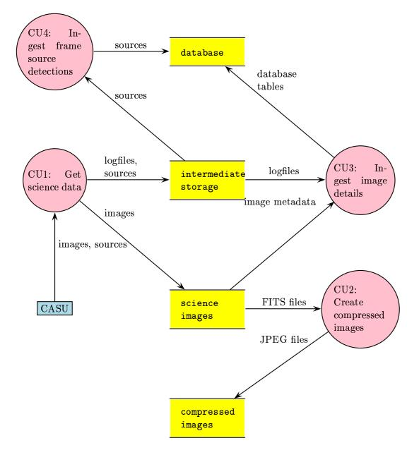
Figure 3: Data flows involved in the data input and ingestion stages
