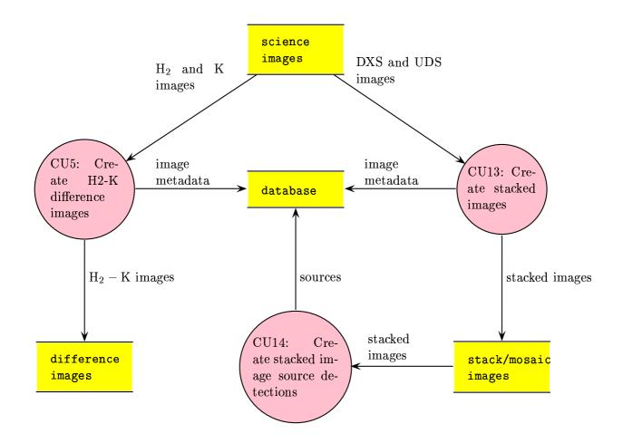
Figure 4: Data flows involved in generating post-ingestion archived data products
