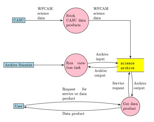
Figure 2: Top level overview of data flows in and out of the WFCAM Science Archive
