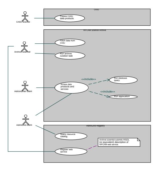
Figure 1: UML use case diagram depicting the functional relationship of the WFCAM science archive with actors and external systems.
